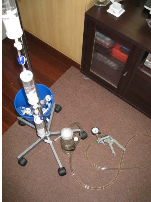
Figure 4: Final arrangement with filter and collection vessel.
